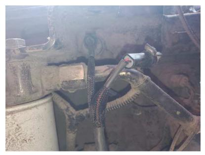
**6)** Connect the red wire with a ring terminal to a constant 12 volt source. Connect the black wire with a ring terminal to a good engine ground. Wiring can be routed over the engine to the Alternator. Note: For RV's, power and ground needs to be connected to the engine, not the house battery system.
