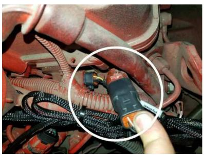
**5)** Continue to the next 2 sets of injector connectors. Repeat Step 4 to connect each pair of injector connectors. Note: The new harness will connect in series between the stock injector plugs and stock wiring plugs. All plugs on the new harness will be connected.
