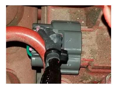
8) Connect the red wire with ring terminal to a +12V constant source, such as the intake air heater grid relay. Connect the black wire with ring terminal to a good Chassis Ground.
