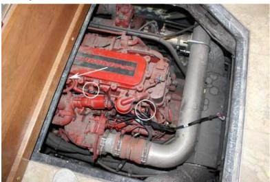
**2)** Unplug all 3 sets of stock injector connectors. Press the release tab on the connector and gently pull the connector apart.
