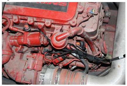
**4)** Locate the first injector connector near the flywheel side of the engine. Plug the female injector connector on the Ag Diesel Solutions module harness labeled "flywheel" into the stock male injector connector. The male injector connector on the Ag Diesel Solutions module harness will plug into the female injector connector.
