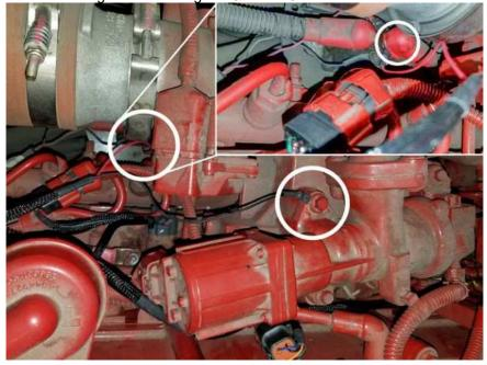
**9)** Plug the Harness into the module. Mount the module with supplied zip ties away from any excessive heat or moving parts. Note: Zip tie the module to the factory wire harness. Mounting the module with the switch connector down will help prevent moisture from collecting into the module connector.
