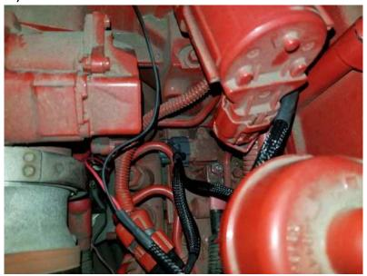
**7)** Plug the Ag Diesel Solutions female MAP sensor connector into the stock male MAP sensor. Plug the Ag Diesel Solutions male MAP sensor connector into the stock female MAP sensor connector.
