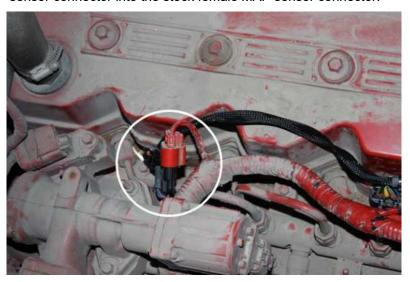
8) Connect Red wire with ring terminal to a +12V constant source. Connect the Black wire with ring terminal to a good Chassis Ground. On the constant +12V of the intake air heater grid relay. Note: Use the engine battery, not the "house" battery.
