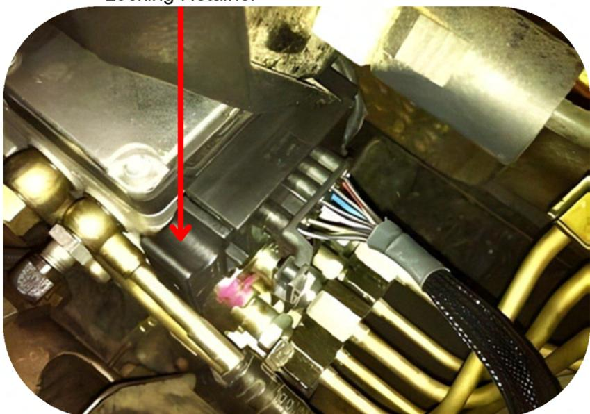
**Step 2)** Slide out locking retainer and remove wiring harness.
