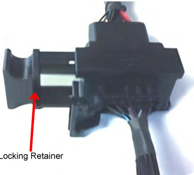
**Step 3)** Plug female connector from module directly into Injection Pump. Plug the male connector from module into the stock harness that was removed from Injection Pump.
