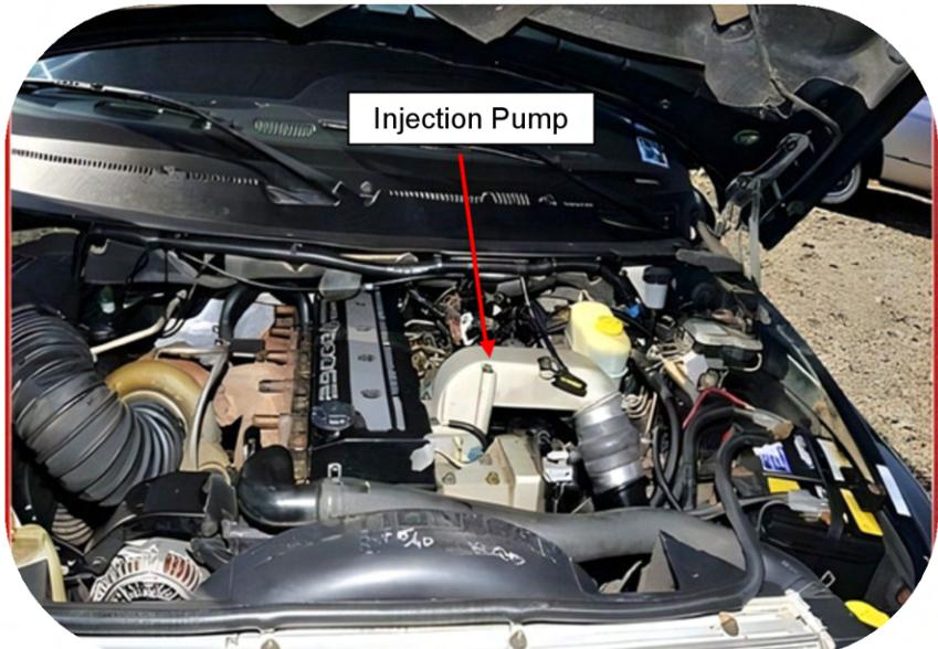
**Step 1)** Locate the injection pump on the driver's side of the engine.
