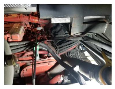
**4)** Locate the first injector connector near the flywheel side of the engine. Plug the female injector connector on the Ag Diesel Solutions module harness labeled "flywheel" into the stock male injector connector. The male injector connector on the Ag Diesel Solutions module harness will plug into the female injector connector.
