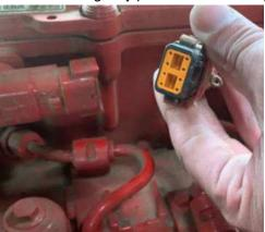
**3)** Route the Module Harness as shown in the picture below. The Module Case will be located closer to the Fan side of the engine.
