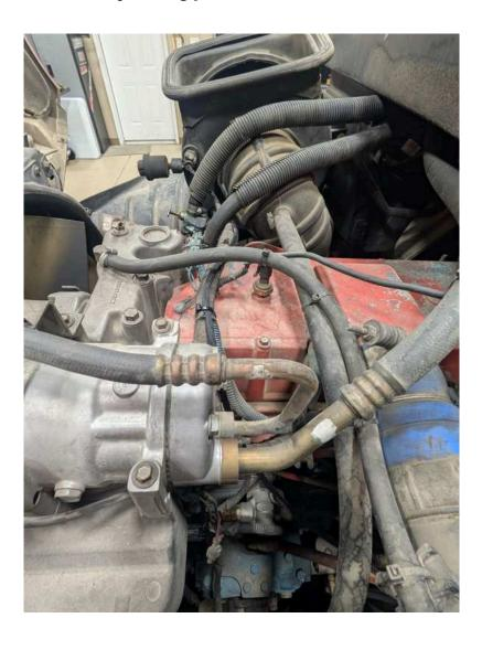
6) Connect Red Wire (12V) to Power on alternator. Connect Black Wire (Ground) to Ground cable bolted to mounting bolt on alternator.
