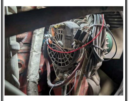
7) Plug the Harness into the module. Mount the module with supplied zip ties away from any excessive heat or moving parts. Note: Zip tie the module to the factory wire harness. Mounting the module with the connector down will help prevent moisture from collecting into the module connector
