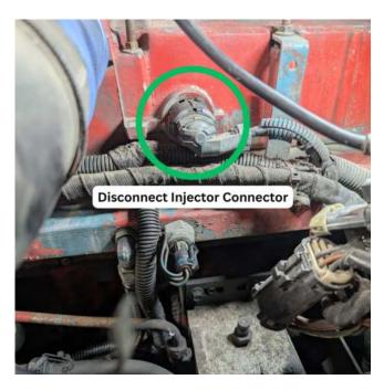
3) Connect the factory injector connector to the Male 13100 injector connector. Connect the female 13100 injector connector to the male injector connector on the valve cover.
