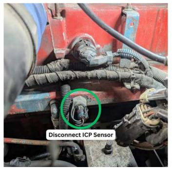
5) Connect the factory ICP connector to the Male 13100 ICP connector. Connect the female 13100 ICP connector to the ICP sensor.
