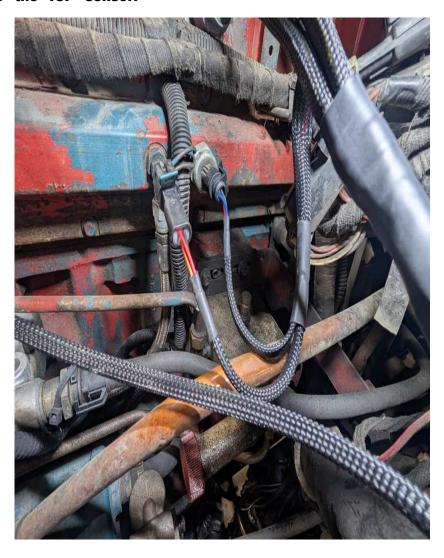
6) Route Power and Ground leads over top of the engine away from heat or any moving parts to the alternator.
