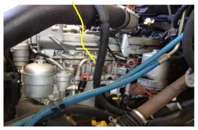
4) For non-egr equipped engines, you can remove a plug in the stock Mercedes Engine cover and route the harness through the opening.
