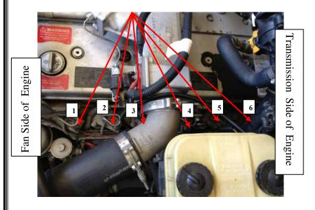
**3)** For EGR equipped engines, route the new harness over the intake toward the "fan-side" of the engine. The harness will route to each one of the 6 Unit Injectors. There is an opening in the Mercedes Cover for the wiring to route.
