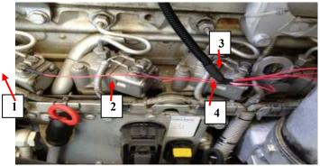
8) Continue routing the wiring toward the transmission-side of the engine.
