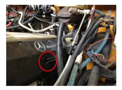
5) Route the module harness wiring in order from 1-8, as shown below. The #1 tag will start at the Unit Injector closest to the engine fan.
