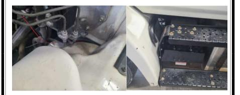
**7)** Install the black wire with the ring terminal to the negative ground battery terminal. Connect the red wire with the ring terminal to the 12 volt battery terminal.
