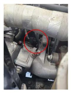
**5)** Plug the male module MAP sensor connector into the stock female MAP sensor connector. Plug the male stock MAP sensor harness into the module female connector.
