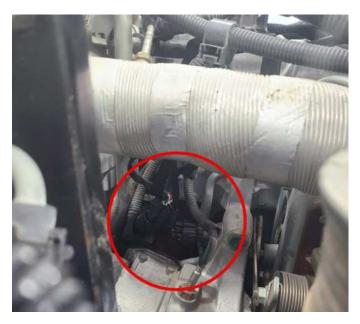
**6)** Route red and black wires with ring terminals behind driver side fender well to battery box under drivers side door.
