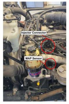
2) Disconnect the stock male injector connector.
