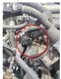
**3)** Plug the male module injector connector into the stock female sensor connector. Plug the male stock injector harness connector into the module female connector.
