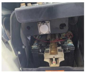
**8)** Mount the module with the provided zip ties in a secure and dry location. Keep away from excessive heat and moving parts.
