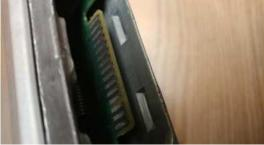
Scrub off the coating using the scotch brite pad provided or a fine sandpaper. The contacts should start to become shiny and metallic copper color. Scrub only until you begin to see a hint of copper. Wipe off any remaining coating with rubbing alcohol or lacquer thinner on a paper towel.
