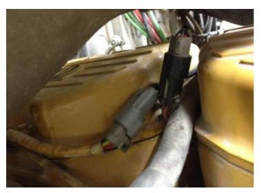
5) Route the power and ground wires to the alternator located on the passenger's side of the engine. Connect the red wire to +12 volts and the black wire to ground.
