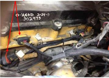
5) Locate the MAP sensor on the driver's side of the engine.
