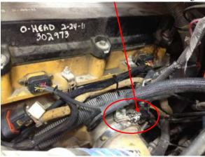
**6)** Disconnect the MAP Sensor. Plug male connector from module into MAP Sensor. Plug stock male connector from the engine harness into the module female connector
