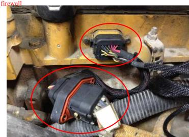
**4)** Follow Steps 2 and 3 for the second injector connector located closest to the engine fan.
