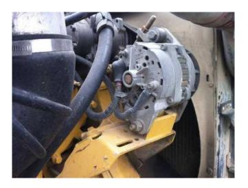
**6)** Plug the harness into the module. Mount the module with supplied zip ties away from any excessive heat or moving parts.
