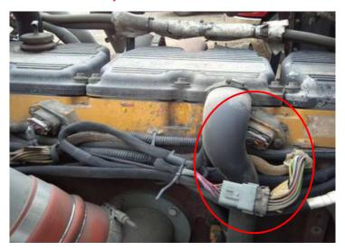
3) Unplug the stock male injector connector located closest to the engine fan. Connect the male connector from the module harness into the injector connector on engine head. Connect the stock male injector connector into the corresponding female harness plug on the module harness. Note: Use the injector connector on the module harness marked "Fan"
