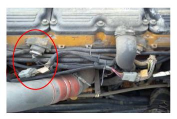
**4)** Disconnect the MAP Sensor. Plug male connector from the module into the stock MAP Sensor on the engine. Plug stock male connector into female connector on module harness. Note: If the MAP Sensor on your engine is rectangle-shaped, then the MAP Sensor Jumpers supplied will not be used. If your MAP Sensor is triangle-shaped, then attach the MAP Sensor Jumpers to the module harness and install as shown below.
