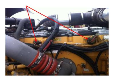
2) Unplug the stock male injector connector located closest to the firewall. Connect the male connector from the module harness into the injector connector on the engine head. Connect the stock male injector connector into the corresponding female harness connector on the module harness. Note: Use the injector connector on the module harness marked "Flywheel".
