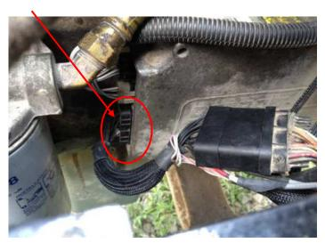
**5)** Locate the 2 injector connectors next to the ECM engine harness and unplug both connectors.
