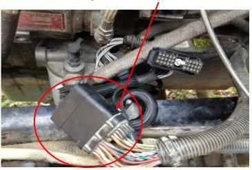
**4)** Connect the male harness into the stock female connector located on the ECM. Tighten the ½" bolt to secure the connector to the ECM
