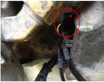
**10)** Plug the harness into the module. Mount the module with supplied zip ties away from any excessive heat or moving parts.
