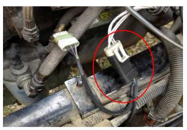
7) Connect the gray injector connector into the stock ECM. It will connect in the lower of the 2 plugs on the ECM.
