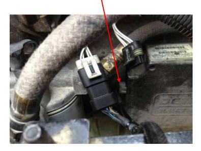
**8)** Plug the stock black female injector connector into the performance module male injector connector.
