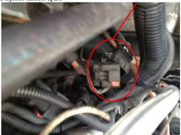
3) Insert the male connector from the module into the male connector on the engine. Plug the male injector connector into the female connector from the module.
