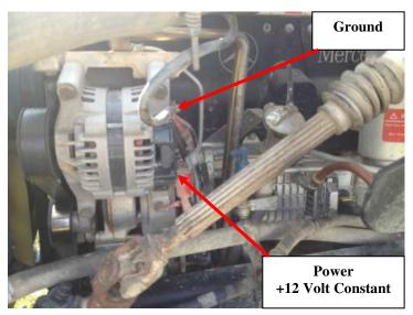
**6)** Plug the Harness into the module. Mount the module with supplied zip ties away from any excessive heat or moving parts. Note: Zip tie the module to the factory wire harness. Mounting the module with the connector down will help prevent moisture from collecting into the module connector
