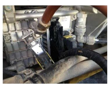
**4)** Connect the Ag Diesel Solutions female harness into the stock female plug located on the engine harness. Squeeze the connector together and then press the locking lever to latch the connector together.
