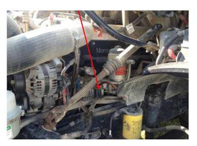
**2)** Disconnect the stock ECM Harness by pushing the Locking Lever down to release. Remove the harness from the ECM.
