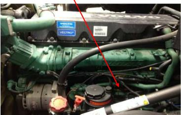
2) Disconnect the stock ECM harness as shown below rotate the yellow locking lever to release. Remove the harness from the ECM.
