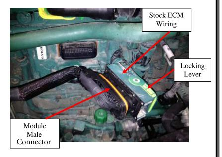
**4)** Plug the module female harness connector into the stock male connector located on the ECM. Press the connector together and then rotate the locking lever to latch the connector to the ECM.
