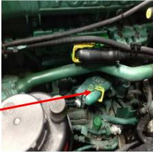
3) Plug the male connector from the module harness into the stock ECM wiring. Squeeze the connectors together and then rotate the locking lever to latch the connectors together.
