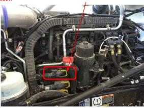
2) Plug the male connector from the module harness into the ECM.
