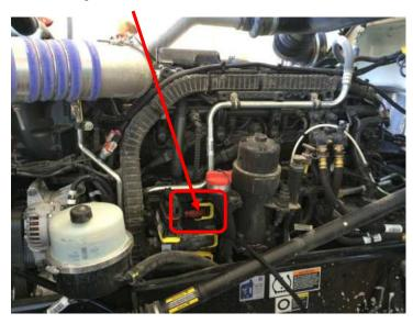
3) Plug the factory male harness into the female connector. Squeeze the connector together and then press the locking lever to latch the connector together.
