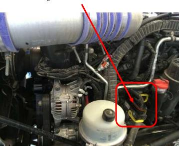
4) Route the power and ground wires to the alternator. The red wire should connect to a +12 volt constant source. The black wire should connect to a good, clean ground.
