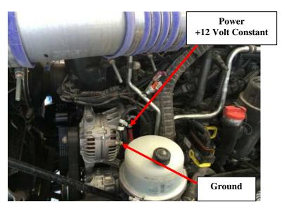
5) Plug the Harness into the module. Mount the module with supplied zip ties away from any excessive heat or moving parts. Note: Zip tie the module to the factory wire harness. Mounting the module with the connector down will help prevent moisture from collecting into the module connector
