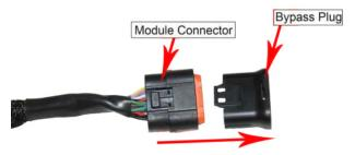
9) Mount the module box in a safe location using the zip ties to secure the wires and module away from any extreme heat and moving parts. Note:Mounting the module with the connector down will help prevent moisture from collecting into the module connector.
