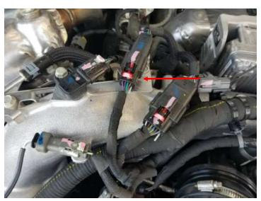
3) The picture below shows the factory fuel sensor disconnected and now you are ready to install the module in it's place.
