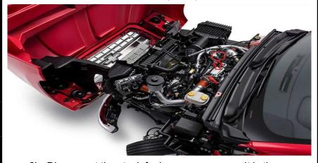
**2)** Disconnect the stock fuel pressure sensor. It is the middle connector shown in the picture. You will have to release the red locking tab and compress the black tab and they will pull apart.
