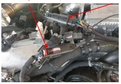
**5)** Unplug the stock MAP sensor. Plug the male MAP sensor from the module into the stock female MAP sensor. Then, connect the stock female MAP sensor into the module harness.
