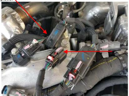
4) Plug the female fuel pressure sensor from the module into the stock male fuel pressure sensor. Then, connect the stock female fuel pressure sensor into the module harness. Note: Make sure you hear the connections "click" then slide the red locking tabs back into place.
