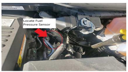
2) Disconnect the stock fuel pressure sensor connector. It is located at the center of the common fuel rail.
