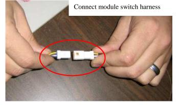
7) Remove the bypass plug from the Ag Diesel Solutions harness, and plug the harness into the module.
