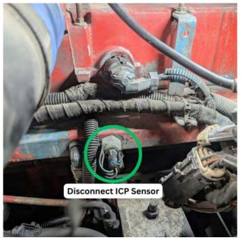
5) Connect the factory ICP connector to the Male 53100 ICP connector. Connect the female 53100 ICP connector to the ICP sensor.
