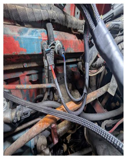
6) Route Power and Ground leads over top of the engine away from heat or any moving parts to the alternator.
