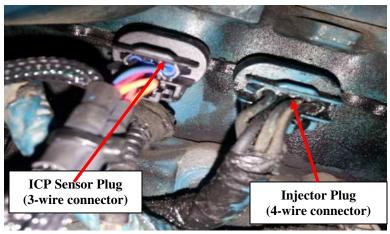
4) Disconnect the stock male ICP Sensor plug and connect it to the female plug on the module harness. Connect the male plug from the module harness into the stock female ICP Sensor.
