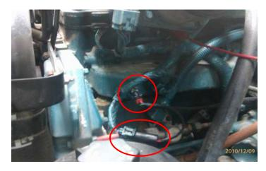
3) In order to locate the ICP Sensor, find each of the 6
