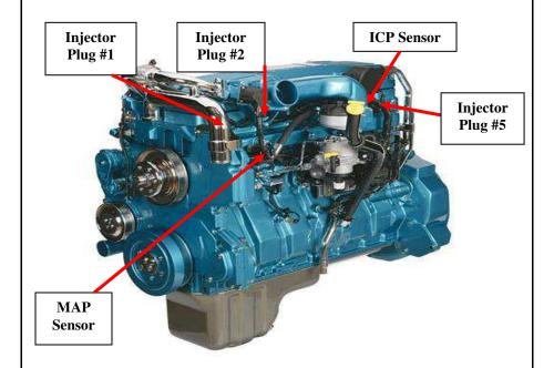
1) Locate the MAP Sensor on the driver's side of the engine. Refer to the picture above for location.
