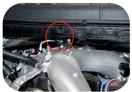
**Step 5)** Locate the MAP sensor on top if the intake manifold and unplug it.
