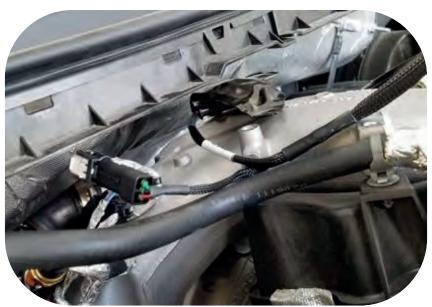
**Step 6)** Plug the male connector from the Ag Diesel Solutions module into the stock MAP sensor. Then plug the male connector from the module into the stock male MAP sensor connector.
