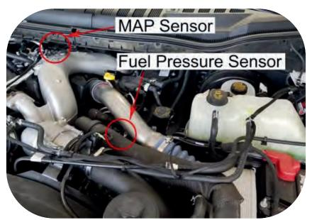
**Step 1)** Locate the fuel pressure sensor on the driver's side of the engine. It is accessible between the Intercooler Tube and Radiator Hose.
