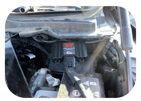
**Step 9)** Mount the module in a safe location using the zip ties to secure the wires and module away from any extreme heat and moving parts.
