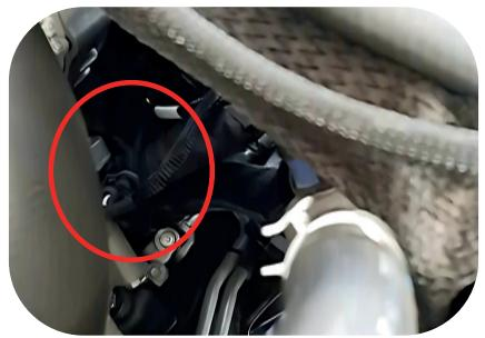
**Step 3)** Plug male connector from module into fuel pressure sensor. Plug the stock connector to the female connector from the module.
