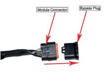
**Step 8)** Remove the bypass plug from the Ag Diesel Solutions harness, and plug the harness into the module.
