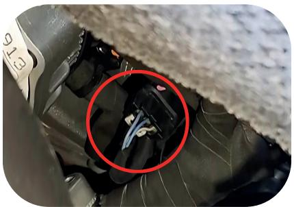
**Step 2)** Unplug the fuel pressure sensor. It is located at the end of the Common Fuel Rail. The Common Fuel Rail runs alongside the valve cover.
