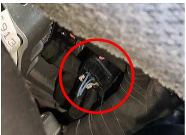
3) Plug male connector from module into fuel pressure sensor. Plug the stock connector to the female connector from the module.
