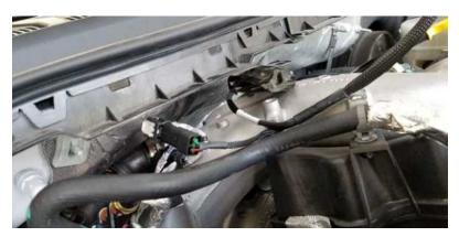
7) Route switch through firewall and plug into module.
