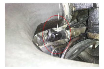
**3)** Plug the male side of module harness into the factory female plug, next plug female side of harness into fuel pressure sensor.
