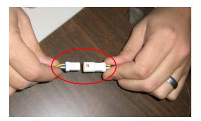
5) Remove the bypass plug from the Ag Diesel Solutions harness, and plug the harness into the module.
