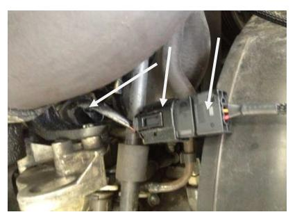
4) Route switch through firewall (optional) and plug into module as shown below.
