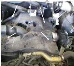
4) Once cover is removed locate Fuel pressure relief valve on back of engine on passenger side.
