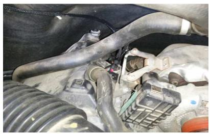
5) Unplug the Fuel pressure sensor. Plug female connector on harness into fuel pressure sensor. Plug factory plug into male side of harness.
