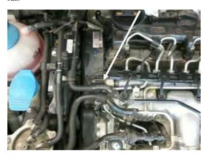
3) Unplug Fuel pressure sensor plug and plug module harness into sensor, next plug factory sensor plug into module harness.
