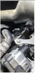
**4)** Plug male Truck Edition fuel pressure connector into the factory fuel pressure sensor. Apply even pressure until connector clicks into place.
