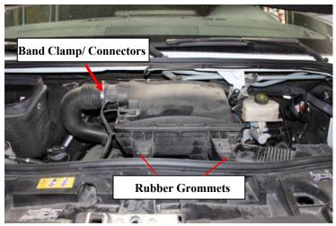
1) Remove the plastic air intake box from center of engine. Unplug two connectors attached to intake box. Release the band clamp connecting to the intake tube and detach the intake air box from rubber grommets.
