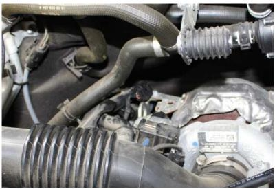
**3)** Unplug the stock fuel pressure sensor connector from the fuel pressure sensor.
