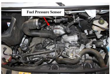
2) With the intake air box removed, locate the fuel pressure sensor at the upper left side of the engine.
