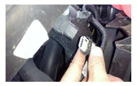
6) Connect the Ag Diesel solution male T-MAP connector to the stock female T-MAP Sensor. Then connect the stock male T-MAP sensor to the female T-MAP connector on module harness.
