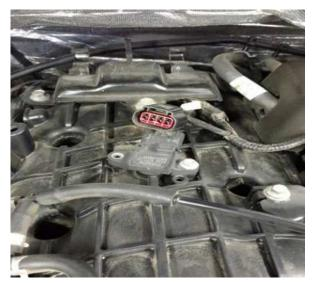
**3)** Connect the Ag Diesel Solutions male MAP sensor into the stock female connector.
