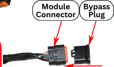
**Make sure to push completely together until connector snaps when using bypass plug.**
