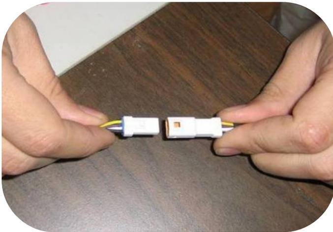
**Step 7)** Route Switch through firewall and plug into module.
