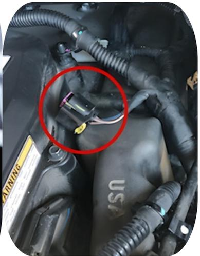
**Step 2)** Disconnect the stock fuel pressure sensor connector. It is located at the center of the common fuel rail.
