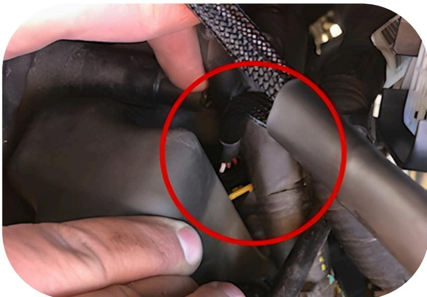
**Step 3)** Connect the male connector from the module into the stock female fuel pressure sensor.
