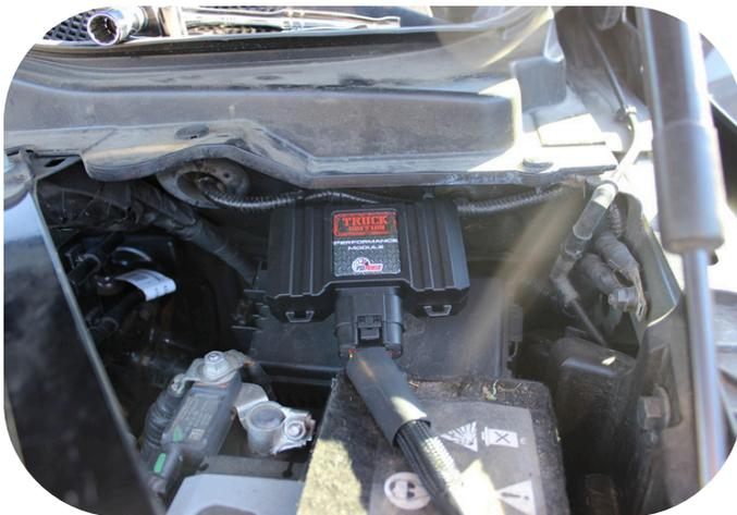
**Step 9)** Mount the module in a safe location using the zip ties to secure the wires and module away from extreme heat and moving parts.
