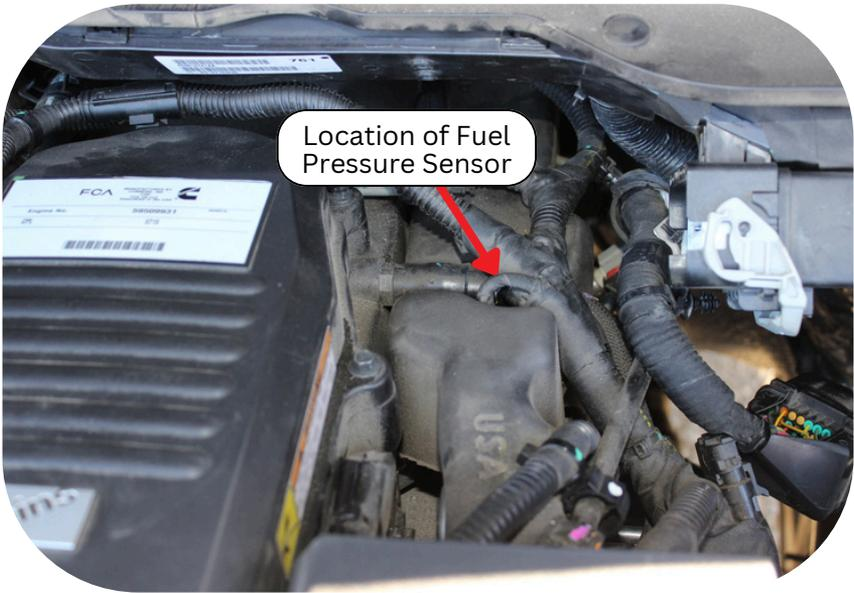
**Step 1)** Locate the Fuel Pressure Sensor on the driver's side of the engine.
