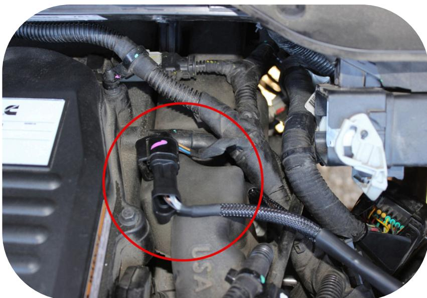
**Step 4)** Connect the stock fuel pressure connector to the female connector from the module.
