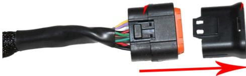
**Step 8)** Remove the bypass plug from the Ag Diesel Solutions harness, and plug the harness into the module.
