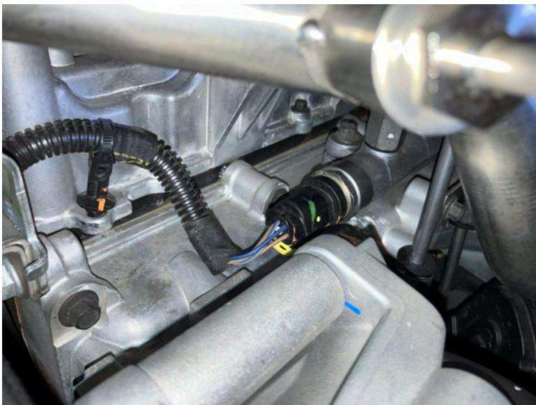
**Step 2)** Disconnect the stock fuel pressure sensor connector. It is located at the end of the common fuel rail.
