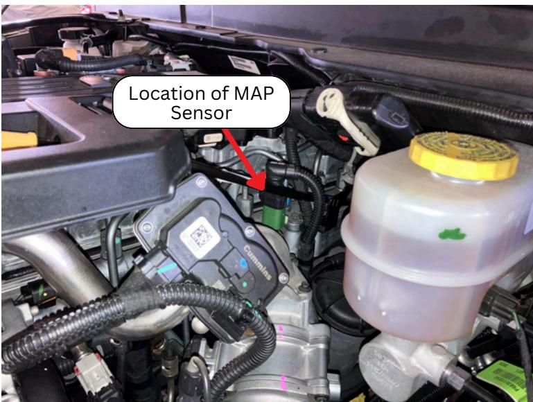
**Step 4)** Locate the MAP Sensor. It is located on the intake manifold on the driver's side of engine.
