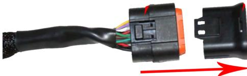
**Step 8)** Remove the bypass plug from the Ag Diesel Solutions harness, and plug the harness into the module.
