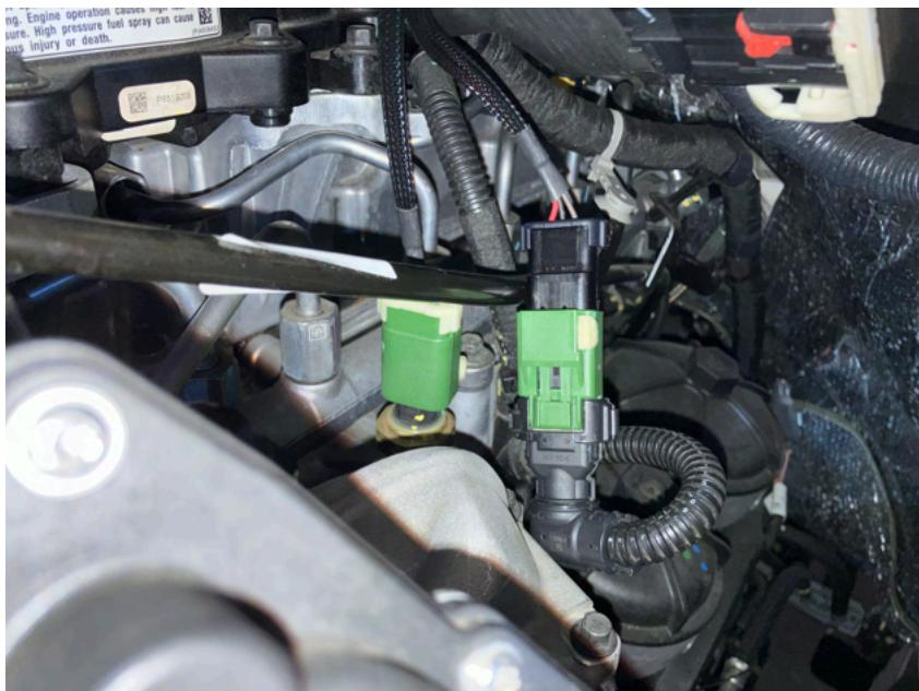
**Step 5)** Disconnect the stock MAP Sensor. Plug the male connector from the module into the stock MAP Sensor. Plug the female connector from the module into the stock wiring harness
