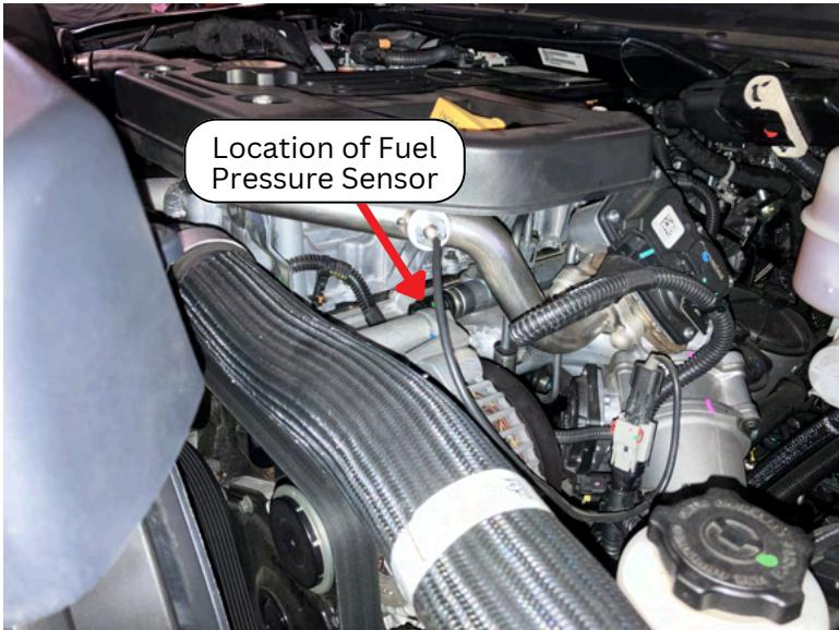
**Step 1)** Locate the Fuel Pressure Sensor on the driver's side of the engine.
