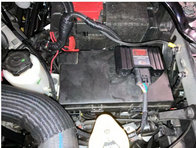
**Step 9)** Mount the module in a safe location using the zip ties to secure the wires and module away from extreme heat and moving parts.
