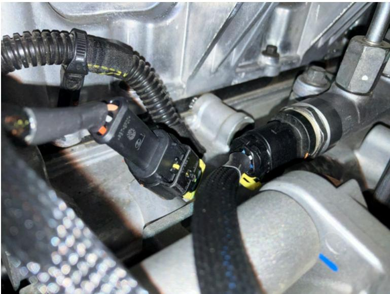
**Step 3)** Connect the male connector from the module into the stock female fuel pressure sensor. Connect the stock fuel pressure connector to the female connector from the module.
