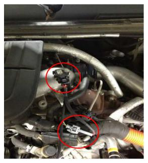
) Route the Switch through firewall and plug into module as shown below
