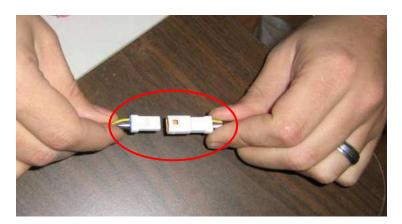
**6)** Remove the bypass plug from the Ag Diesel Solutions harness, and plug the harness into the module.
