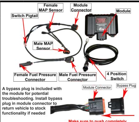
Make sure to push completely together until connector snaps when using bypass plug.
