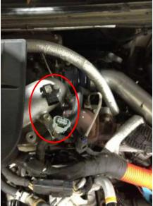
4) Plug the male MAP Sensor connector from the module harness into the Stock MAP Sensor. Plug the female MAP Sensor connector into the Stock MAP Sensor male connector.
