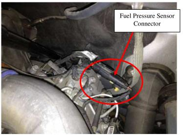
2) Plug the Female Connector from the module into the Stock Duramax male connector. Plug the Stock Duramax female connector to the male connector from the module. The fuel pressure plugs are located closest to the module case on the new harness.
