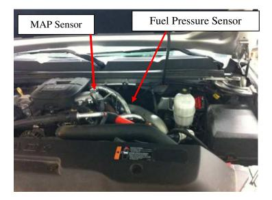
1) Locate Fuel Pressure Sensor connector on the driver's side of the engine and disconnect. It is mounted to the valve cover close to the firewall.
