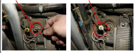
4) Plug the Female Connector from module into the Fuel Pressure Sensor.
