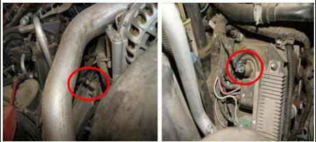
2) Disconnect the Fuel Pressure Sensor.
