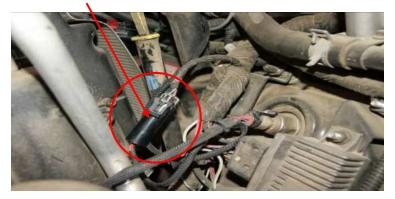
6) Locate the Map sensor on the passenger side of the engine and disconnect it. It is located next to the engine oil fill cap.
