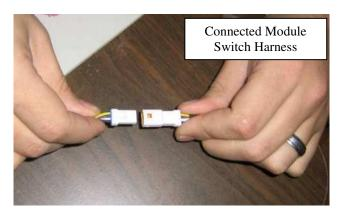
Remove the bypass plug from the Ag Diesel Solutions harness, and plug the harness into the module.
