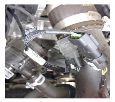
Remove the bypass plug from the Ag Diesel Solutions harness, and plug the harness into the module.
