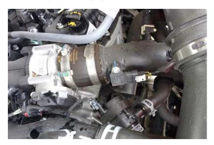
**6)** Utilize the portion of the ADS harness labeled T-MAP. Connect the ADS Female connector to the T-MAP Sensor. Then connect the ADS Male connector to the Factory Female T-MAP Sensor connector.
