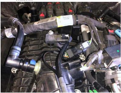
**5**) Disconnect the stock male T-MAP Sensor connector from the T-MAP Sensor.
