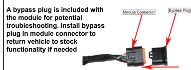
Make sure to push completely together until connector snaps when using bypass plug.
