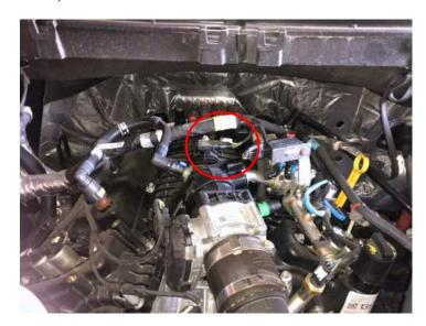
**4)** Utilize the portion of the Ag Diesel Solutions harness labeled MAP. Connect the male connector to the MAP Sensor. Then connect the ADS female connector to the stock male MAP Sensor connector.
