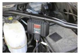
9) Connect module switch harness. Based on preference, the module switch can be secured in the engine compartment near the module or it can be routed into the cab. If mounting in the cab, route the Switch through the firewall and connect to the module harness.
