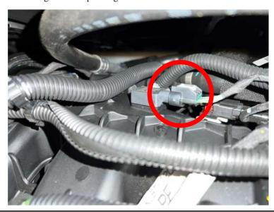
**3)** Utilize the portion of the Ag Diesel Solutions harness labeled MAP. Connect the male connector to the MAP Sensor. Then connect the ADS female connector to the stock male MAP Sensor connector..
