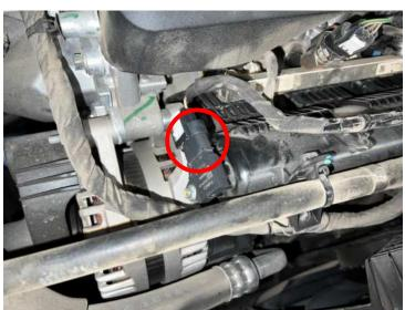
**3)** Utilize the portion of the Ag Diesel Solutions harness labeled MAP. Connect the male connector to the MAP Sensor. Then connect the female connector to the stock male MAP Sensor connector.
