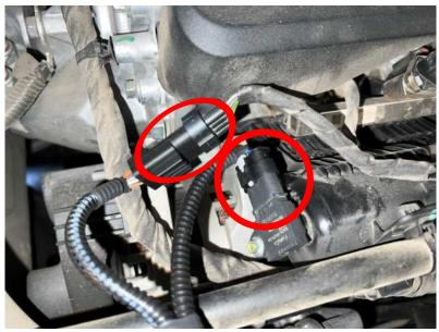
**4)** Disconnect stock T-MAP sensor connector by pulling back on locking tab and squeezing the connector release tab.
