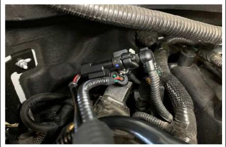
5) Disconnect the stock male MAP Sensor connector from the MAP Sensor.
