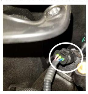
**4)** Utilize the portion of the Ag Diesel Solutions harness labeled MAP. Connect the male connector to the T-MAP Sensor. Then connect the ADS female connector to the stock male T-MAP Sensor connector.
