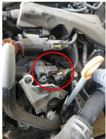
**3)** Connect the ADS female MAP connector to the factory MAP sensor. Connect the ADS male MAP connector to the factory female MAP sensor connector.
