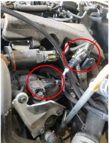
**4)** Disconnect the factory female T-MAP sensor connector from the T-MAP sensor by pressing down on the release tab and pulling out of the sensor.
