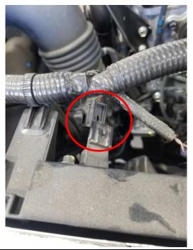
**5)** Connect the ADS female T-MAP connector to the factory T-MAP sensor. Connect the ADS male T-MAP connector to the factory female T-MAP sensor connector.
