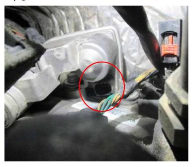
**3)** Plug Female Connector from module into TTVA connector and plug Male connector from module into TTVA harness.
