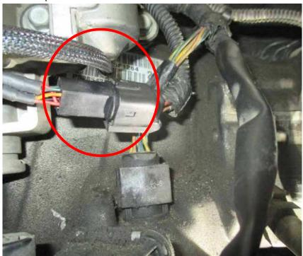
4) Connect module switch harness. Based on preference, the module switch can be secured in the engine compartment near the module or it can be routed into the cab. If mounting in the cab, route the Switch through the firewall and connect to the module harness.
