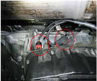
**4)** Connect module switch harness. Based on preference, the module switch can be secured in the engine compartment near the module or it can be routed into the cab. If mounting in the cab, route the Switch through the firewall and connect to the module harness.
