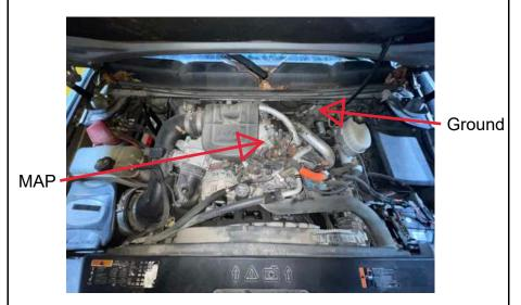
2) Unplug MAP connector from the unit. Plug Female Connector from module into MAP connector and plug male connector from module to MAP harness.
