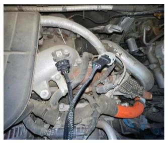
**3)** Unbolt the groundstrap. Add the ground wire to groundstrap bolt. Fasten the nut back on the bolt.
