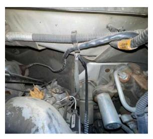
**4)** Locate the transmission plug near the passenger side, between the front and rear tires.
