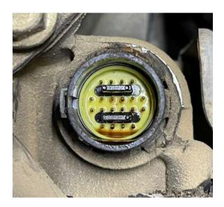
7) Plug Female Connector from module into Transmission connector and plug Male connector from module to Transmission harness.
