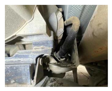
**6)** Remove any residual transmission fluid from the connector and plug to ensure clean connection.
