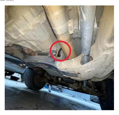
**5)** Route harness to transmission plug, keeping away from heat sources and rotating parts. Ziptie any hanging parts of the harness. Unplug transmission harness from the transmission plug.
