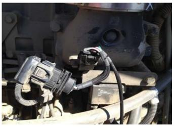
**7)** Connect Red wire with ring terminal to a 12V constant source (i.e. alternator)
