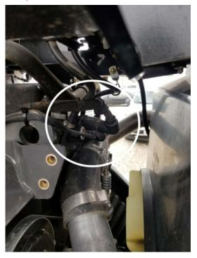
**5)** Unplug the stock female MAP sensor by depressing the release tab and pulling back on connector.
