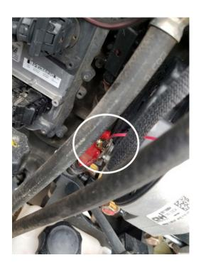
**8)**Connect the Black wire with Ring Terminal to a good chassis ground. Note: Make sure ground surface is clean metal to metal contact. Even if surface underneath painted components seems clean, abrasive cleaning or alternate location is recommended.
