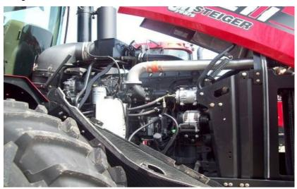
**2)** Unplug the stock injector connector from the front side of the cylinder head. To loosen, rotate the outer shell of the connector counter-clockwise.
