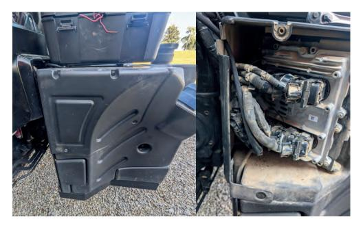
2) Unplug the stock #8 ECM connector by rotating the locking lever on top of the connector towards the right. Note: The #8 ECM plug is located on the top left as you face the ECM. You will need to remove the other three plugs to its right to gain access.
