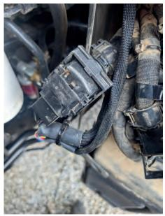
**5)** Mount the red power wire to the intake air heater grid relay, +12 volt constant source and the ground wire to one of the AC compressor mounting bolts.
