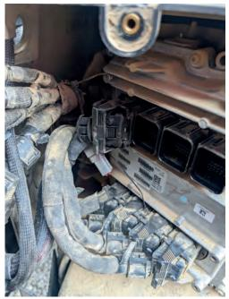
**4)** Plug the stock male connector located on the engine harness into the female connector on the module harness. Gently push the connectors together while you rotate the locking lever to latch the connectors together.
