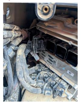
3) Plug the male connector from the Ag Diesel Solutions module into the ECM. Note: The locking lever on the module will slide in to lock the connector in place. The orientation is the same as the stock connector.
