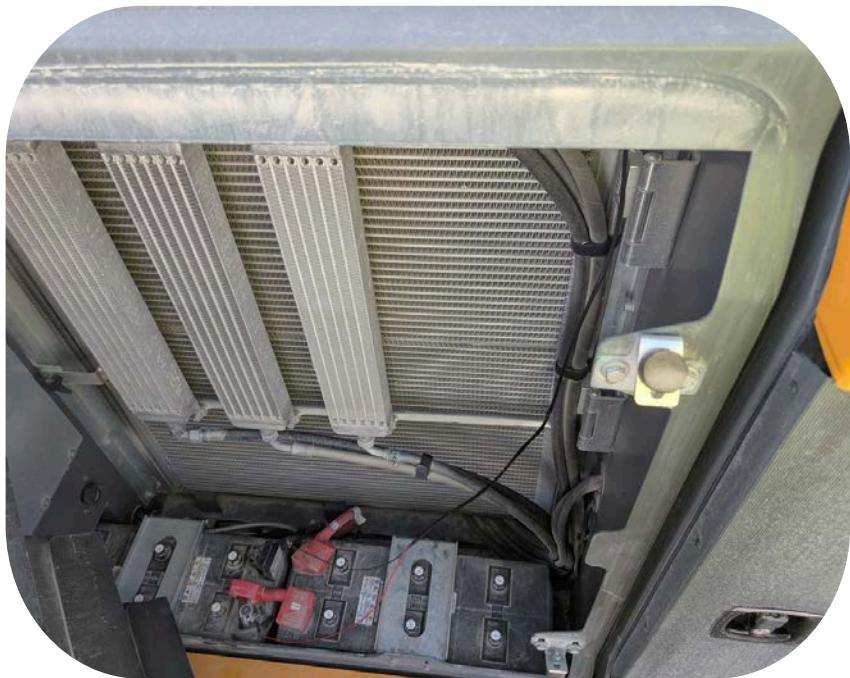
**Step 5)** Once you have located the batteries, measure them with a multimeter to find 12V. **\*\*THIS MODULE NEEDS TO BE HOOKED UP TO 12 VOLTS ONLY\*\***
