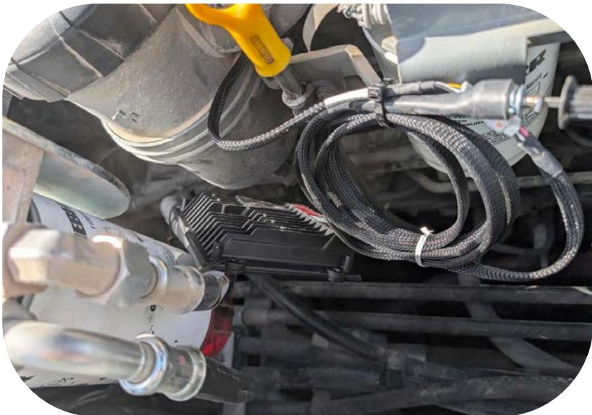
**Step 10)** Connect the module to the harness. Secure and mount the module away from heat or moving parts. Connect the rotary switch to the harness and mount where desired.
