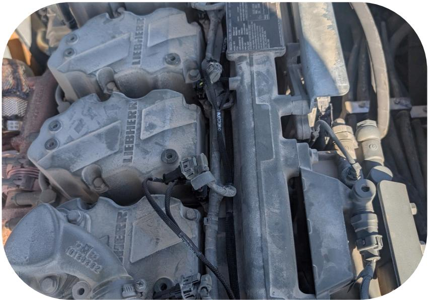
**Step 3)** Unhook the factory female injector connectors from all 6 injectors. Connect them to the AG Diesel Solutions harness accordingly. Connect the AG Diesel Solutions female connectors back into each injector accordingly.
