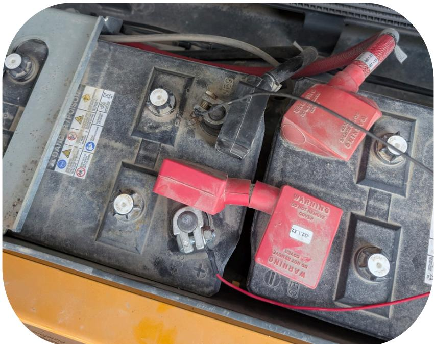
**Step 9)** Connect the **Red Wire (Constant 12V) to 12V on the battery**. Connect the Black Wire (Ground) to the negative on the battery.
