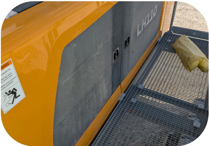
**Step 4)** Locate the machines engine batteries. They are located behind the unmarked engine cover on the “Drivers Side” of the machine.
