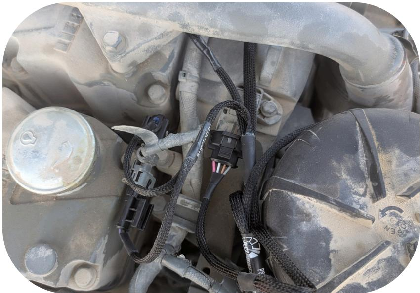
**Step 2)** Unhook the factory female map sensor connection from the map sensor and connect it to the AG Diesel Solutions harness. Connect the Ag Diesel Solutions female connector back into the map sensor.
