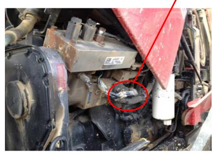
**2)** Connect the male connector from the module into the stock female plug. Connect the female connector from the module into the stock male connector.
