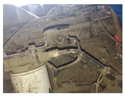
**4**) Plug the male MAP sensor connector from the Ag Diesel Solutions harness into the stock female map sensor. Connect the female MAP sensor connector from the module harness into the stock male MAP sensor connector.
