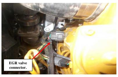
**6)** Unplug the stock EGR valve connector. Press and hold the release tab on the connector and gently pull the connector apart.
